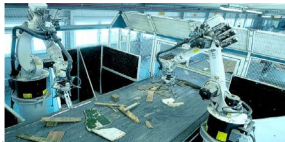
Figure 3. ZenRobotics Recycler, the first robotic waste sorting system to reclaim raw materials
